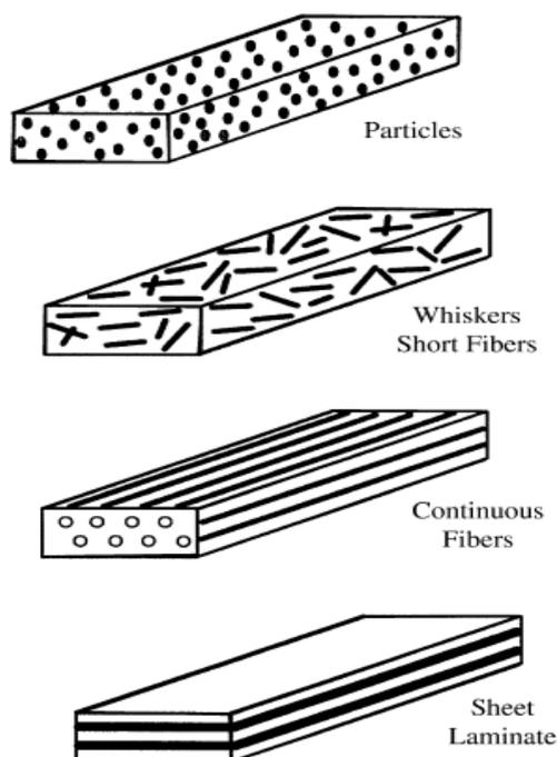
Fig.1 Different types of Metal Matrix Composites [7]
